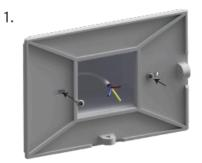
Mount the back plate to the wall box using 2 screws and feed the wires through the opening.
